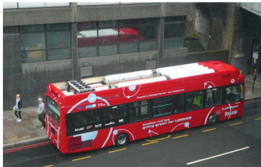
Figure 10: Image showing rooftop gaseous hydrogen storage (Pocard & Reid, 2016)
